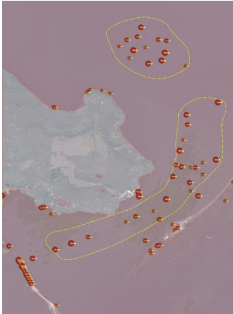
Fig. 4 The Sentinel-2 input image fragment with results of ships detection by spectral features using the developed method
