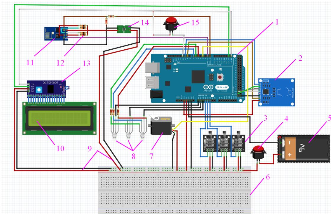
Legend: 1 – microcontroller board (central control) Arduino; 2 – RFID module; 3 – sensors (Hall or touch); 4 – power button; 5 – Li-Po Battery 9 V; 6 – circuit board; 7 – servo motor; 8 – LED (RGB); 9 – breadboard Dupont jumper wires; 10 – LCD screen; 11 – Wi-Fi module; 12 – resistors; 13 – I2C module; 14 – DC converter 3V/5V; 15 – start button.
