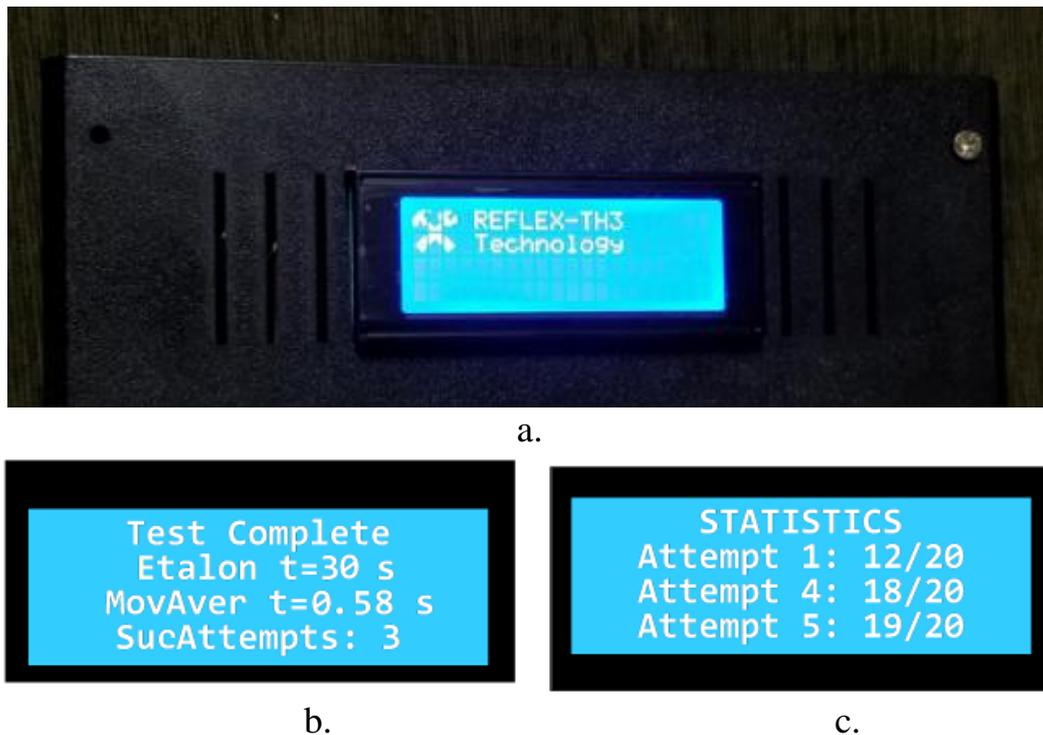
Fig. 8 Device Logo (a) and test results after training: b – move average time; c – test statistics (unsuccessful / successful actions of each attempt)
