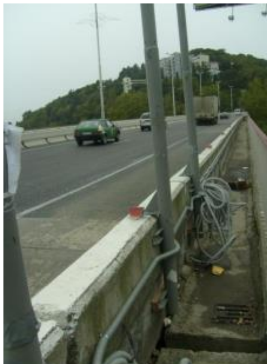
Fig. 4 Special supports to fix strain gauges-photodetectors
