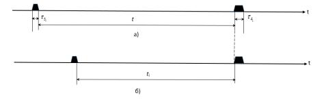
Picture 8. Time diagrams of operation of the device without deformation of the bridge span (a) and after deformation (b).
