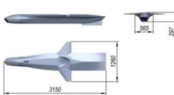
Fig. 3. General view of the aircraft "Mini-Flight - M"
