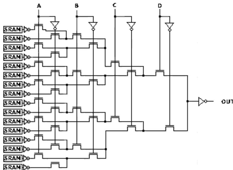
Fig.1 – Logic cell - a 4-input LUT FPGA
