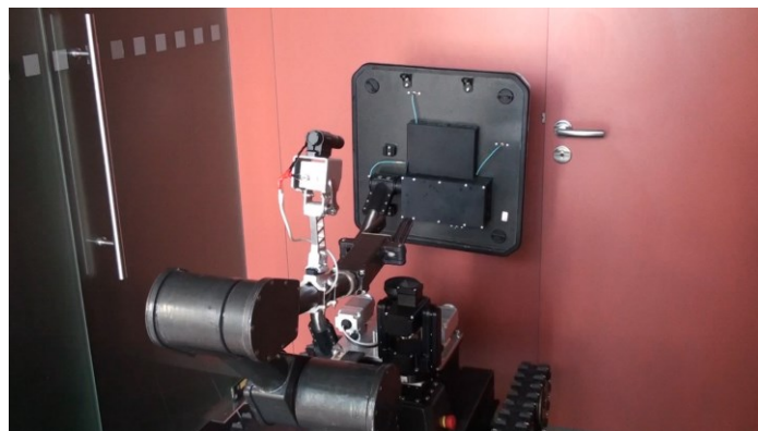
Fig. 6 Photo of bioradar sensor mounted on robot in action.
