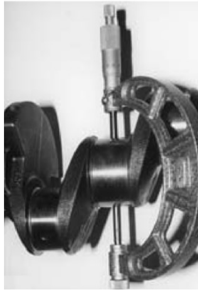
Fig. 2 Measuring a bearing with micrometer [4]
