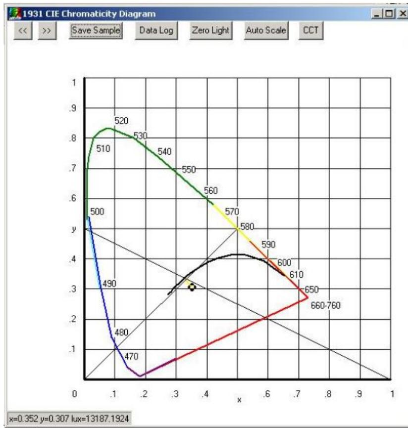
**Fig. 7.** Result showing spectral and photometric characteristics of our luminaire for desired CCT – 4400K, measured CCT = 4450K,  $I_{white} = 350\text{mA}$ ,  $I_{blue} = 185\text{mA}$ , luminous flux  $Y_{\Sigma} = 1404\text{lm}$
