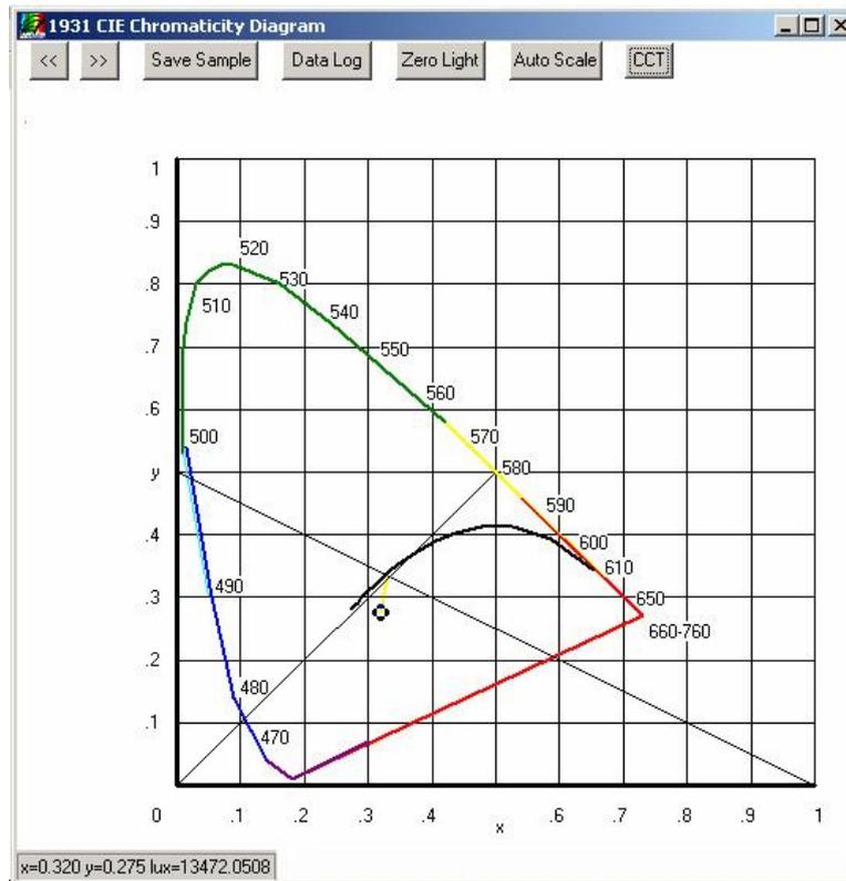
**Fig. 8.** Result showing spectral and photometric characteristics of our luminaire for desired CCT – 6500K, measured CCT = 6490K,  $I_{white} = 350\text{mA}$ ,  $I_{blue} = 285\text{mA}$ , luminous flux  $Y_{\Sigma} = 1432\text{lm}$
