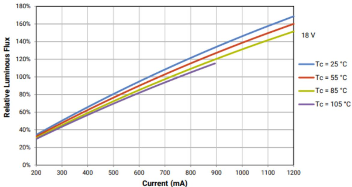
Fig. 3. Relative luminous flux as a function of operating current for CREE CXB1512 2700K, 80CRI LED modules [6].
