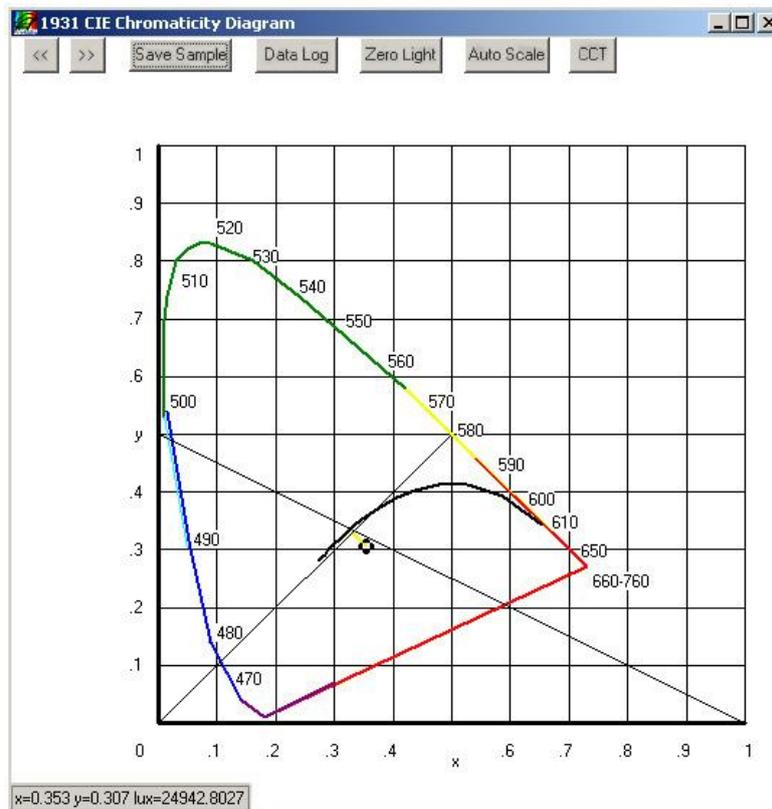
**Fig. 7.** Result showing spectral and photometric characteristics of our luminaire for desired CCT – 4400K, measured CCT = 4369K,  $I_{white} = 700\text{mA}$ ,  $I_{blue} = 360\text{mA}$ , luminous flux  $Y_{\Sigma} = 2666\text{lm}$
