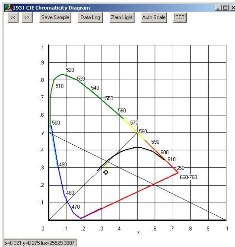
**Fig. 9.** Result showing spectral and photometric characteristics of our luminaire for desired CCT – 6500K, measured CCT = 6435K,  $I_{white} = 700\text{mA}$ ,  $I_{blue} = 632\text{mA}$ , luminous flux  $Y_{\Sigma} = 2709\text{lm}$
