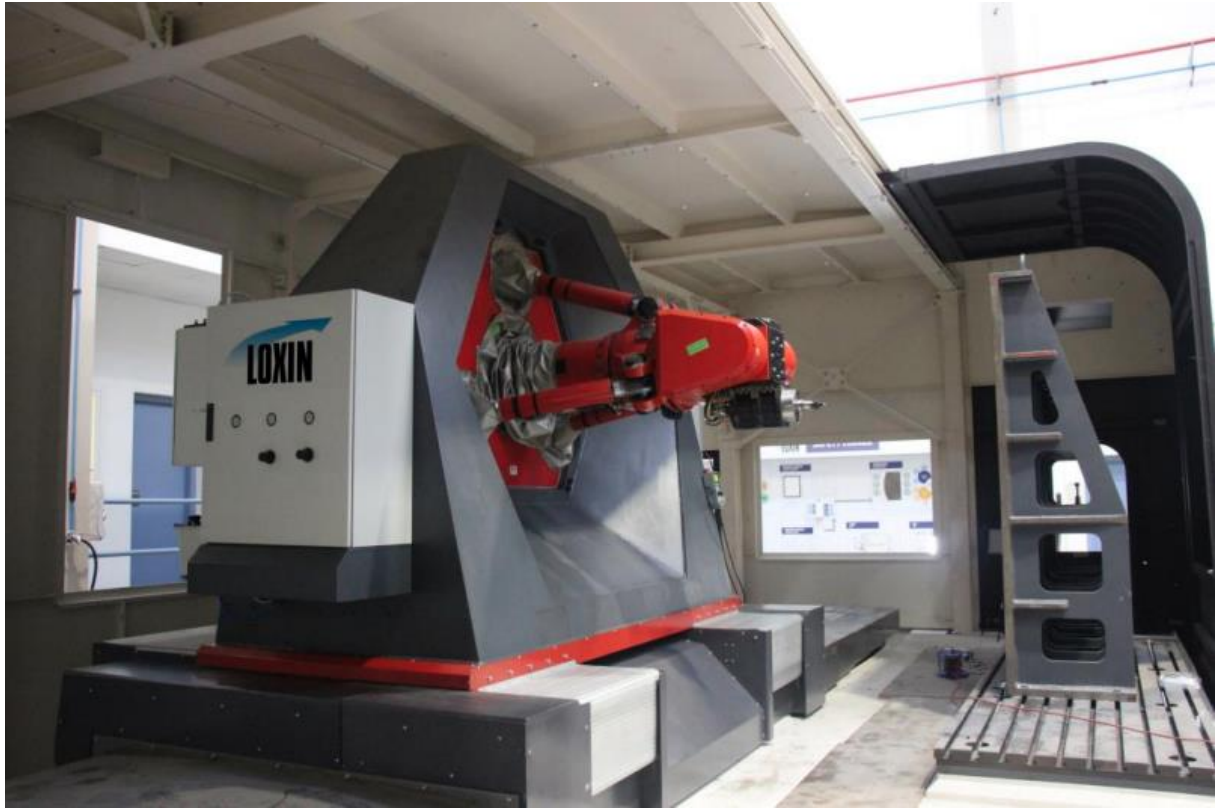
Fig. 2 HyPrint Technology showcasing its additive and subtractive manufacturing capabilities. [8]
