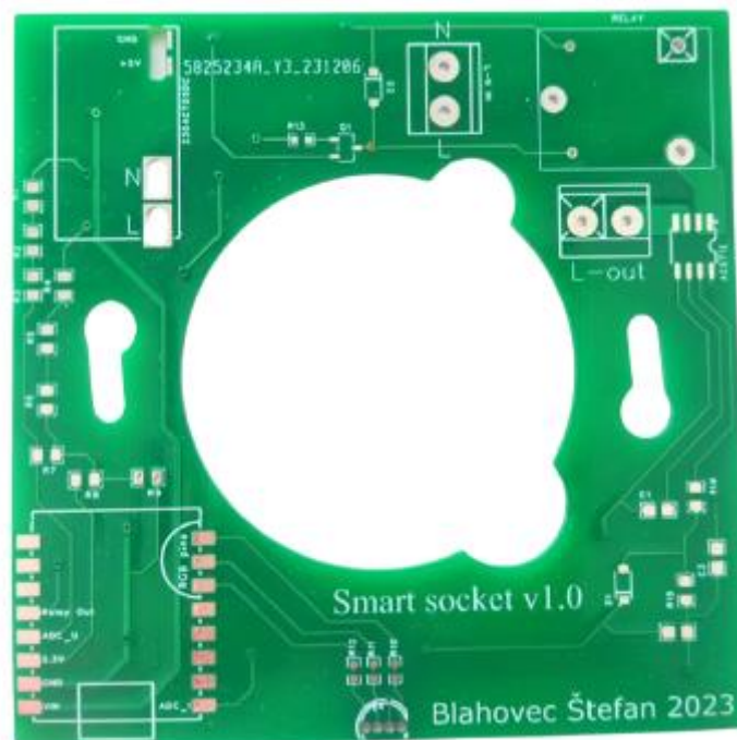
Fig. 3 Final PCB of the device
